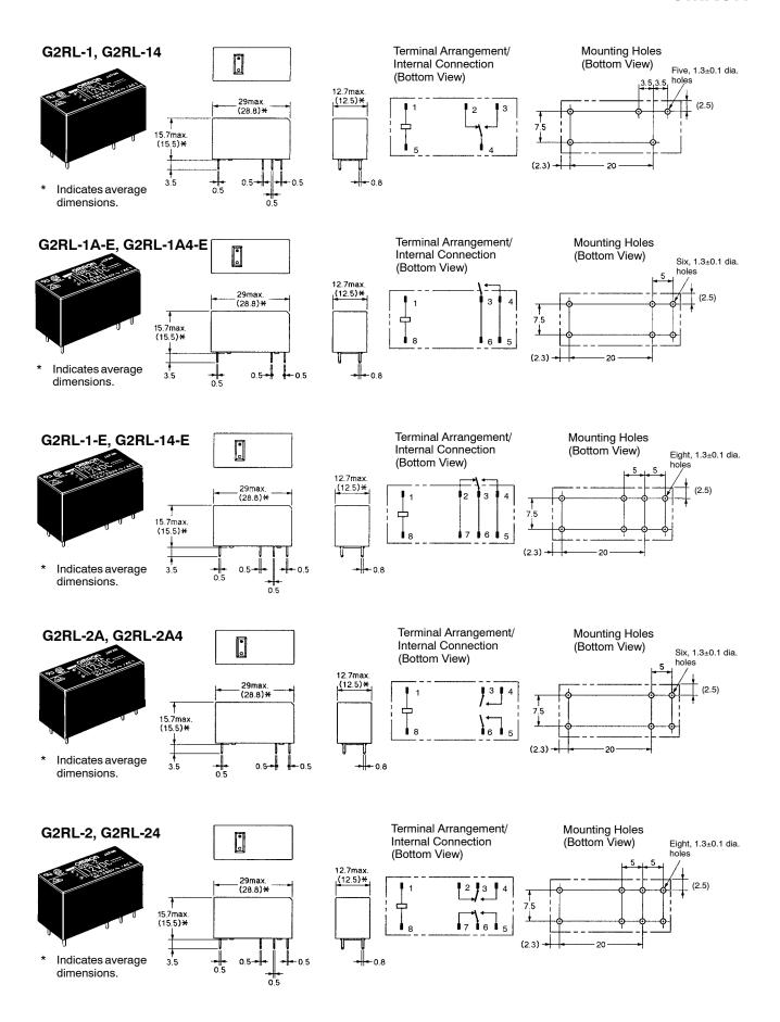
ALL DIMENSIONS SHOWN ARE IN MILLIMETERS. To convert millimeters into inches, divide by 25.4
